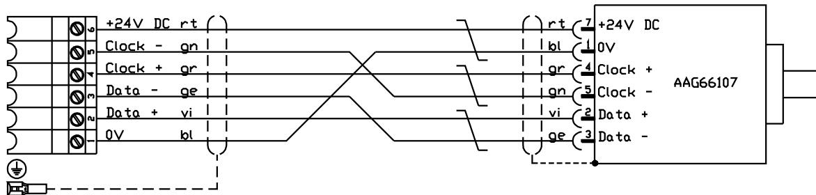
**Please note:** Only use a sheathed pairwise connection cable. Do not put the cable near power current wires. If possible, put the screening up at both sides.
