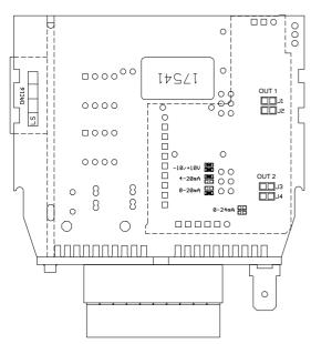
If you want to change the signal level, the device has to be opened. The case can be opened in the middle using a screwdriver. On the solding side of the largest printed circuit board two solding bridges for every analog output, i.e. the analog output 1(OUT1) and 2 (OUT2), are located, which are named J1 to J4 in the drawing to the right. J1 and J2 are used to adjust the signal level for output 1 and J3 and J4 to adjust the output level for output 2.
