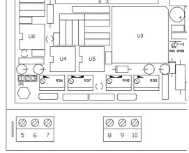
has to be known with great accuracy. It should be in the range of 15 to 20 mA. Now choose the menu in which this value is displayed in the device (CamCon). You are able to increase this displayed value by turning to the left at the R36 (input 1) or R39 (input 2) or de-crease it by turning to the right. Set the now present current or it's corresponding value and seal the potentiometer with sealing wax. At the potentiometers atR37 and R40 no configuration can be done while being under current.
