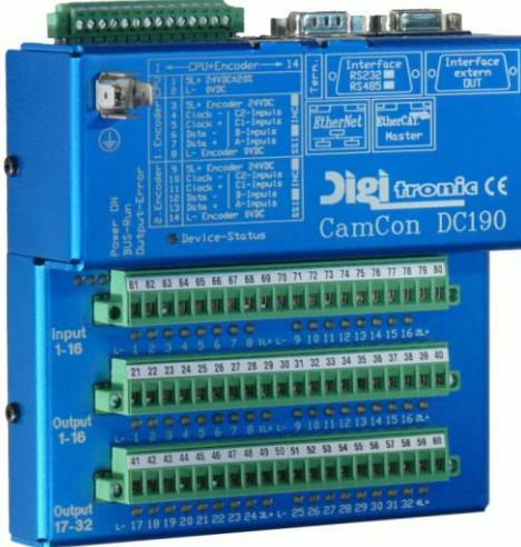
**Attention:** The second Ethernet connection of the DC190 named EtherCAT is fixed a EtherCAT master and must never be connected to the PROFINET become.
