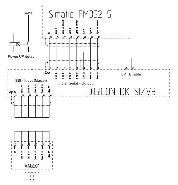
In this example, the DK SI/V3 is connected to a Simatic FM352-5 cam controller. This controller can not provide a release or enable signal for the DIGICON.
