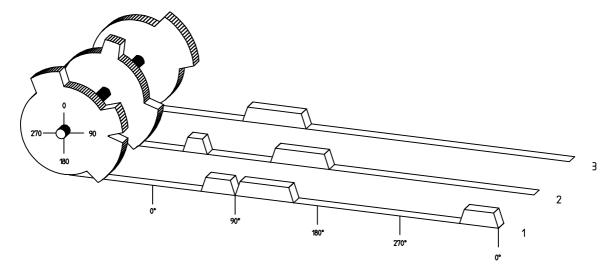
Diagram: Principles of a Cam Switch Unit
