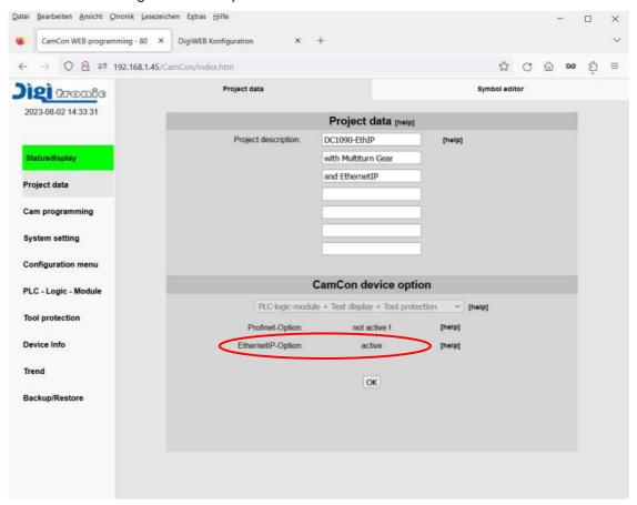
Now you can configure the CamCon DC1090 completely on this WEB - page as it is written in the manual or you can fully configure the DC1090 by the ControlLogix CPU PLC via the DC1090/190 Program TAGs.
