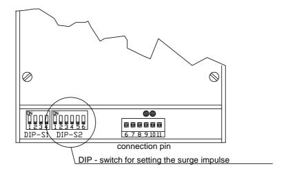
You can set up to eight different overload amplification times for each channel that are adjusted according to the following table.
