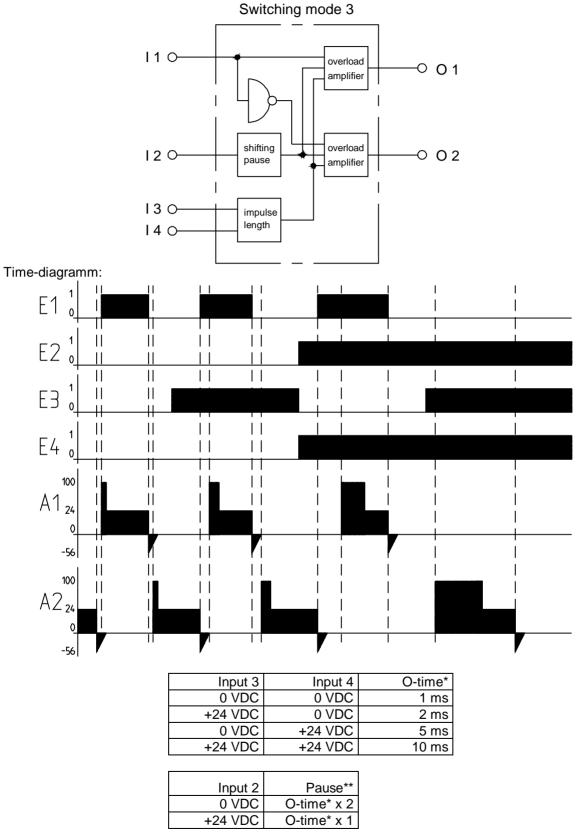
\*O-time: Duration of the overload amplification impulse
