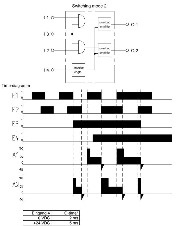
In the switching mode 2 eatures an enabling input I3 (AND - Linkage).
