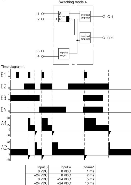
\*O-time: Duration of the overload amplification impulse
