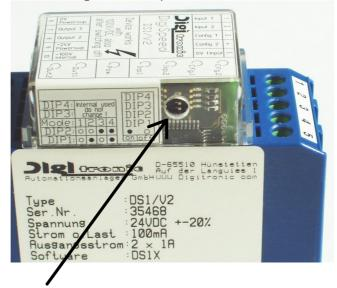
To adjust the dip-switch use a small screwdriver or an bent paper clip.
